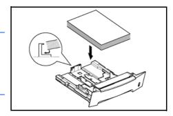
Do not load paper above the triangle mark located on the width guide.
